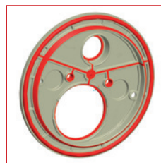
Intelligent solution – squirted sealings: the plate support is manufactured in a 2-component die-casting process. Direct injection moulding ensures that the joints remain perfectly watertight.
