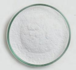
Krion® Solid is mainly composed of high purity white mineral (ATH). This gives the material hardness and resistance, and a unique feel.
