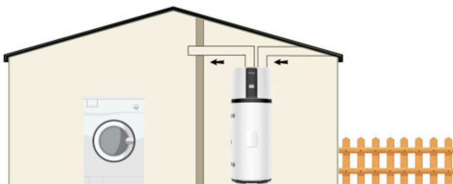
Installation with 2 ducts to the outside
