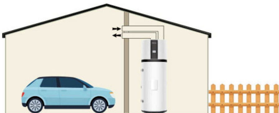
Installation with 2 ducts to an unheated room >15\text{m}^2
