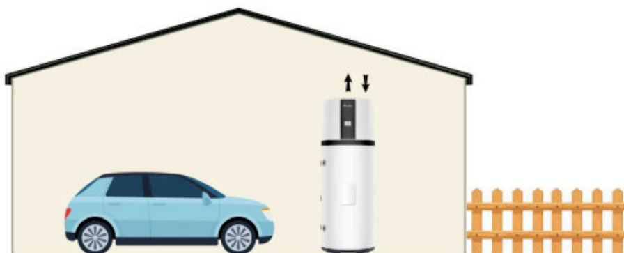
Installation in an unheated room >15\text{m}^2
