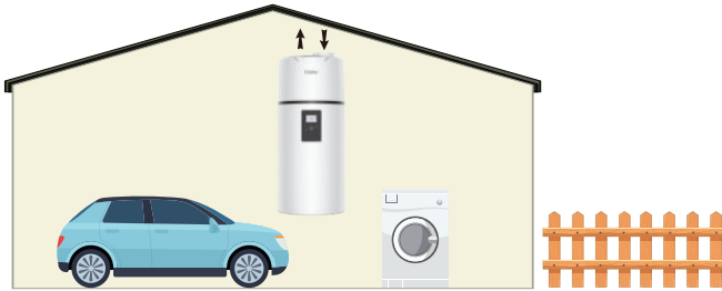
Garage or laundry room (without ducts)
